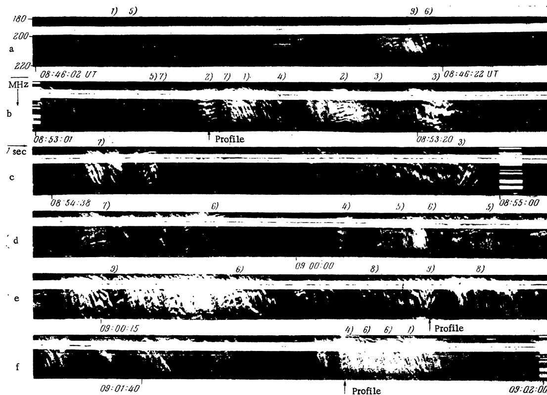
Fig. 4. Microstructure pulsations of the event of July 3, 1974 on the high-resolution spectrograph. Numbers above spectra denote the different types of bands in emission and absorption described in the text.
